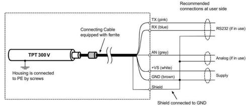
If the user intends to employ his own connecting cable, it is recommended to equip this cable with a ferrite near the sensor. A suitable type is Würth #74271112.
