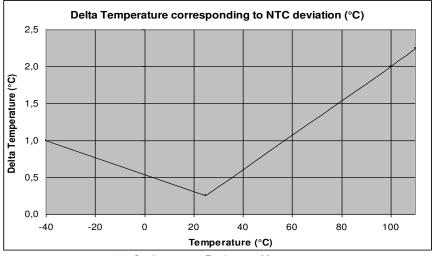
0.1°C tolerance on Resistance Measurement
