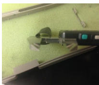
INCORRECT ID TUBING IS STRETCHED
