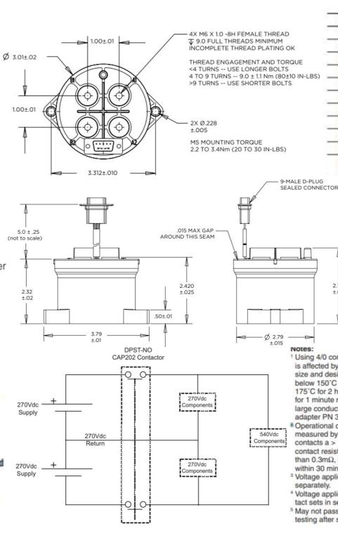
2.72 + 02 1 Using 4/0 conductor. Current rat is affected by attached conducted size and design. Keep terminals below 150°C max, continuous, 175°C for 2 hours max. and 200 for 1 minute max. For mounting large conductors, request termi adapter PN 3-1618396-7. Operational contact resistance measured by millivolt drop acro contacts a > 100A current. Initia contact resistance may be high than 0.3mΩ, but will drop below within 30 mins. max.
