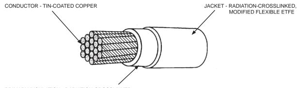
PRIMARY INSULATION - RADIATION-CROSSLINKED, MODIFIED FLEXIBLE ETFE COLOR - LIGHT GREEN
