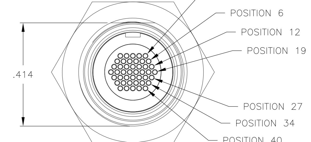
1 CONNECTOR BODY AND JAM NUT MATERIAL: 6061-T6 ALUMINUM, ELECTROLESS NICKEL PLATED PER SAE-AMS-C-26074 OR SAE-AMS-2404E
