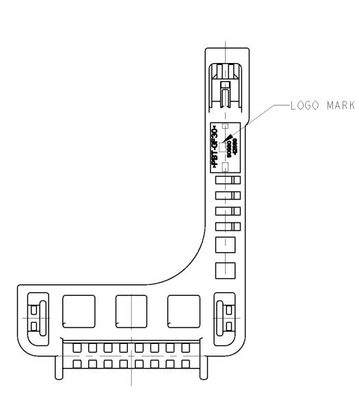
MATING CONNECTOR IS: TYCO ELECTRONICS P/N:1747140
