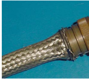
Figure 5. Trimming the Excess Braid
