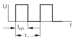
$$df = \frac{t_{on}}{t_{cyc}} \times 100 \text{ (%)}$$
