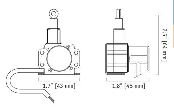
Just like the SM1, the SM2 is the perfect sensing solution when tight space is an issue. With its rugged compact design, handy mounting bracket and a 40-inch electrical cable for easy signal connection, the SM2 is the perfect solution for the OEM and single piece users alike.
