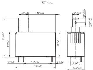
Terminal dimensions: Coil-Terminal:  $0.5 \pm 0.025$ Contact-Terminal:  $0.5 \pm 0.01 \times 0.8 \pm 0.05$
