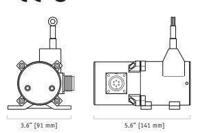
The PT8420 with its 4-20 mA feedback signal, is ideal for monitoring the stroke of a hydraulic cylinder and other applications requiring position data acquistion in harsh environments.
