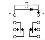
CONTACT RATING: LOW LEVEL TO 1A 28 VDC RESISTIVE 100,000 OPERATIONS
