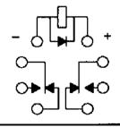
CONTACT RATING: LOW LEVEL TO 1A 28 VDC RESISTIVE 100,000 OPERATIONS
