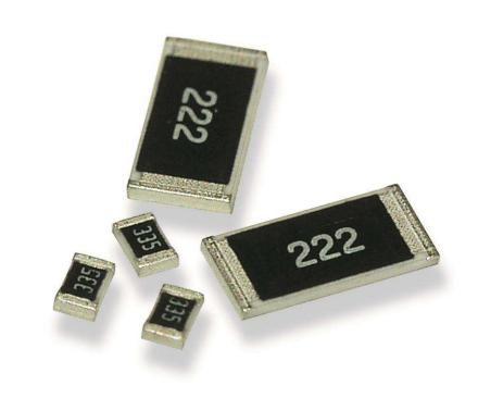
The resistive element is screen printed and fired, and a passivation layer added. Each resistor is trimmed to tolerance by laser. The pre-scribed tile is then broke into strips, the end plating fired on, and the strips broken into individual components. Final termination finish is electroplated matte Sn over a Ni barrier layer.
