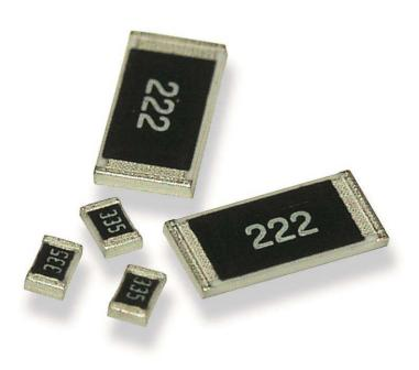
The resistive element is screen printed and fired, and a passivation layer added. Each resistor is trimmed to tolerance by laser. The pre-scribed tile is then broken into strips, the end plating fired on, and the strips broken into individual components. Final termination finish is electroplated matte Sn over a Ni barrier layer.
