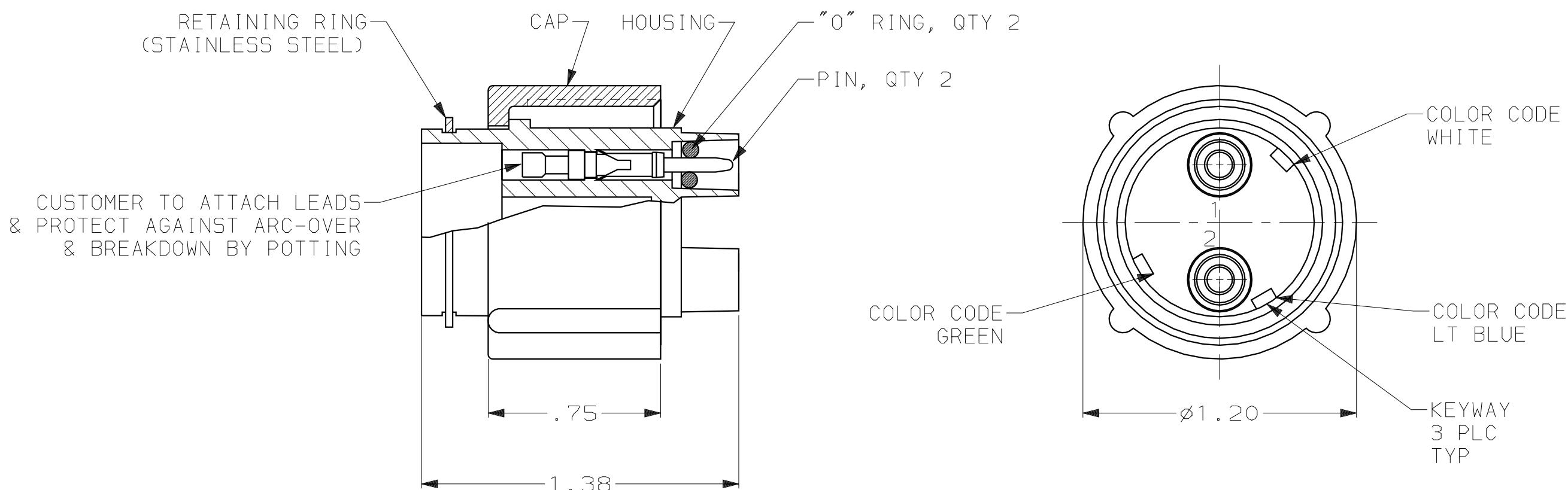
1. PLUG ASS'Y WILL WITHSTAND WITHOUT BREAKDOWN 27 KVDC PIN TO PIN & 27 KVDC PIN TO GROUND WHEN MATED WITH RECEPT.
