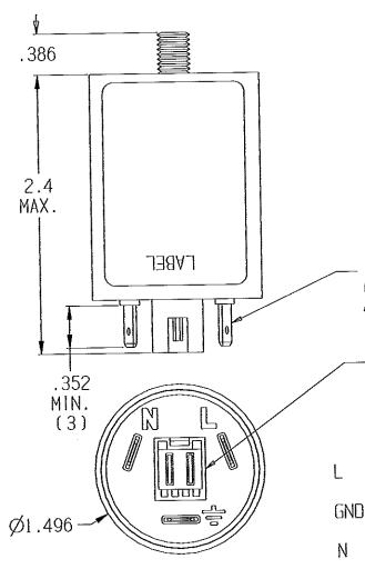
.250 x 0.032 PREINSULATED ULTRA FAST TERMINAL [ACCEPTS T.E. P/N 3-350819-2 (#16 TO #14 AWG WIRE)] APPLICATION SPECIFICATION 114-2123. (3 PLACES)
