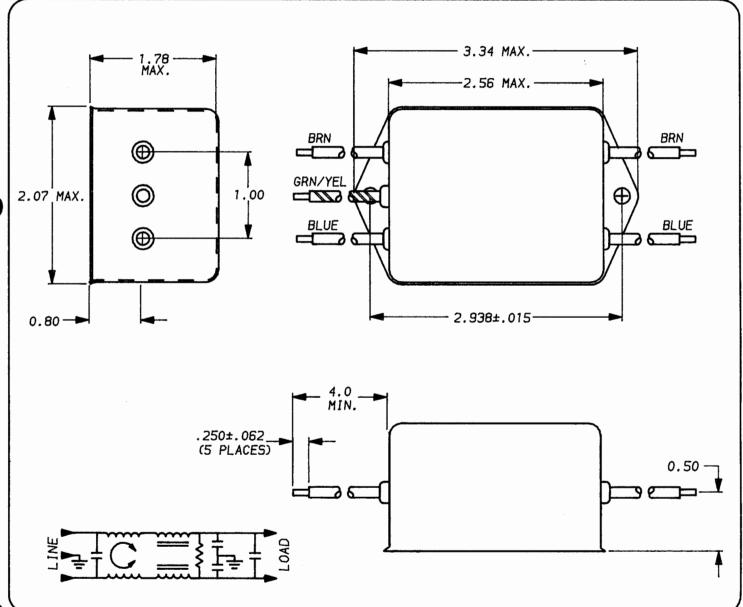
50n - 50n (MINIMUM) INSERTION LOSS UNLESS OTHERWISE SPECIFIED, TOLERANCE TO BE ±.025 FREQUENCY 01 015 02 05 15 .5 1. 2 5 10 20 30 MHz MATERIAL & FINISH: AS SUPPLIED COMMON This document is proprietary to CORCOM INC. and is not to be reproduced nor used for manufacturing purposes except on CORCOM'S prior written consent. 25 25 27 36 47 47 43 45 45 45 45 45 ď₿ DIFF 2 18 43 68 **7**5 75 72 70 65 62 60 **d8**
