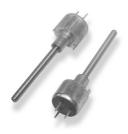
A very popular range is this 13mm diameter spindle operated potentiometer family. The LC1 Series has a cermet resistance element. This technology provides excellent electrical and thermal stability, reliability, low noise and long life, to meet most professional or military applications for small size potentiometers. Recent changes have meant that the LC type is no longer released to BS CECC specification.
