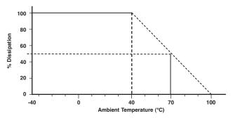
Dissipation as a function of temperature.
