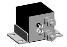
The FCA-150 series relay is a polarized, single-side stable design, where the flux from a permanent magnet provides the armature holding force in the deactivated state, and its flux path is switched and combined
