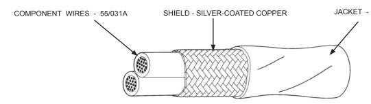
JACKET - LOW OUTGASSING, RADIATION-CROSSLINKED, MODIFIED ETFE
