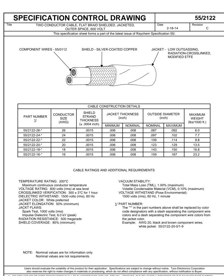
1/ COLORS AND COLOR CODE DESIGNATORS SHALL BE IN ACCORDANCE WITH MIL-STD-681. HOWEVER, DUE TO LENGTH LIMITATIONS OF THE RAYCHEM PART NUMBER, AN ALTERNATIVE COLOR CODE MAY REPLACE MIL-STD-681 COLOR CODE DESIGNATORS. (EXAMPLE: "901/902..." MAY BE REPLACED BY "AXXX".) OTHER CODES AND SUFFIXES MAY BE ADDED TO THE PART NUMBER, AS NECESSARY, TO CAPTURE ANY ADDITIONAL REQUIREMENTS IMPOSED BY THE PURCHASE ORDER.
