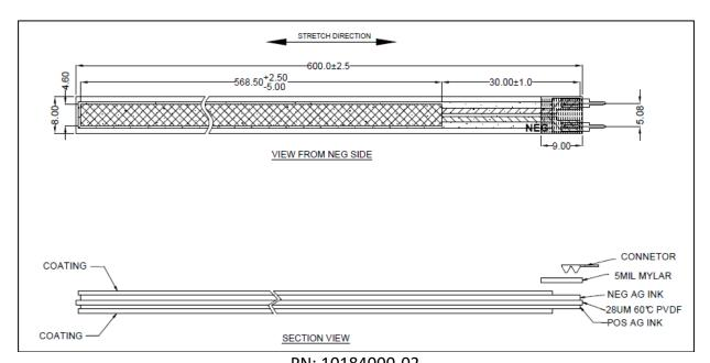
PN: 10184000-02 Capacitance Range: 7.12~11.19 nF Dissipation <=0.030
