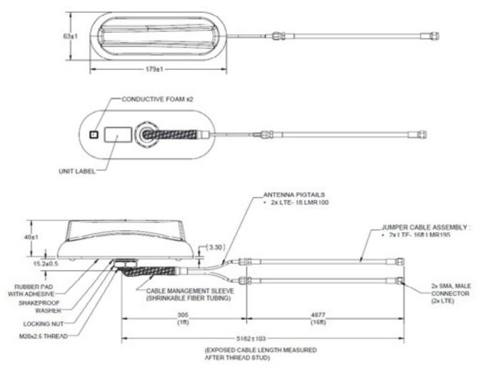
The Gar antenna can create an IP67 water-tight seal when installed on vehicles. Certain vehicles such as a Ford Explorer Interceptor have more narrow roof ridges that are tightly spaced together. For this type, vehicle special adapters are available. See parts **BKIT-VFX69383-001** (between ridges installation) and **BKIT-VFX69383-003** (atop ridge installation) for product details.
