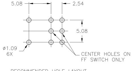
RECOMMENDED HOLE LAYOUT TOLERANCE ±0.05 UNLESS OTHERWISE NOTED
