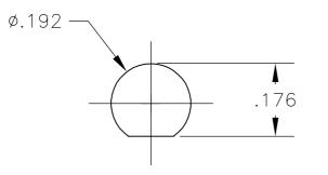
RECOMMENDED HOLE LAYOUT TOLERANCE ±.002 UNLESS OTHERWISE NOTED
