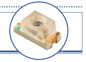
The OP522 is an NPN silicon phototransistor mounted in a miniature SMT package. The device incorporates an integral molded lens which enables a narrow acceptance angle and higher collector currents than devices without lenses. This device is packaged in a 1206 size chip carrier that is compatible with most automated mounting equipment. The OP522 is mechanically and spectrally matched to the OP250 series infrared LEDs.
