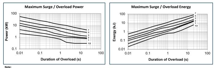
Mounted on a 0.53°C/W heatsink with 5m/s forced air cooling, air temperature 25°C. Single pulse or low repetition rate, such that mean power ≤ 10% of rated power. ΔR ≤ 5%
