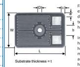
Fixing hole is located centrally except on WSHR1/2 where the dimension from the edge by the terminations to the mounting hole centre is 16.68mm.
