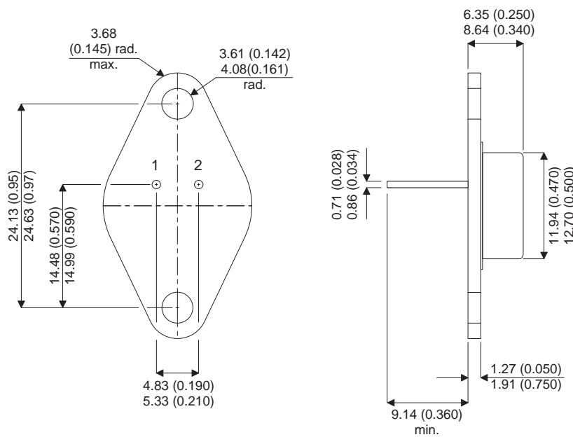
**Bipolar NPN Device in a
