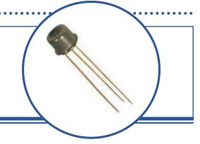
The OPF420 is a low noise silicon PIN photodiode mounted in a low cost package for fiber optic applications. It offers fast response at moderate bias and is compatible with LED and laser diode sources in the 800-1000 nm wavelength region. Low capacitance improves signal to noise performance in typical short haul LAN applications.
