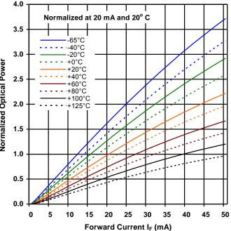
Optical Power vs I<sub>F</sub> vs Temp
