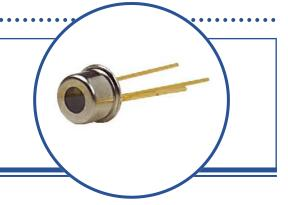
The OPF320 series fiber optic transmitters are high performance devices packaged for data communication links. This transmitter is an 850 nm GaAlAs LED and is specifically designed to efficiently launch optical power into fibers ranging in size from 50/125µm up to 200/300µm diameter fiber. Multiple power ranges with upper and lower limits are offered which allows the designer to select a device best suited for the application.
