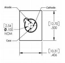
DIMENSIONS ARE IN INCHES AND [MILLIMETERS].
