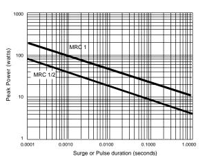
Note: Use for repetitive pulses where the average power dissipation is not to exceed the component rating at  $70^{\circ}\text{C}$ . Surge handling capacity for low-repetitive surges may be significantly greater than shown above.
