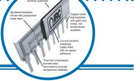
The IRC 4700 Series is the ultimate combination of precision performance, reliability, and long term stability in a low profile,
