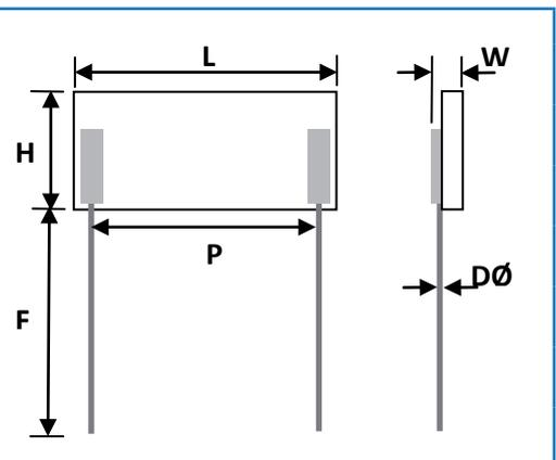
Note 1: Termination pitch dimension P is measured between the lead centres at 1mm from the resistor body.
