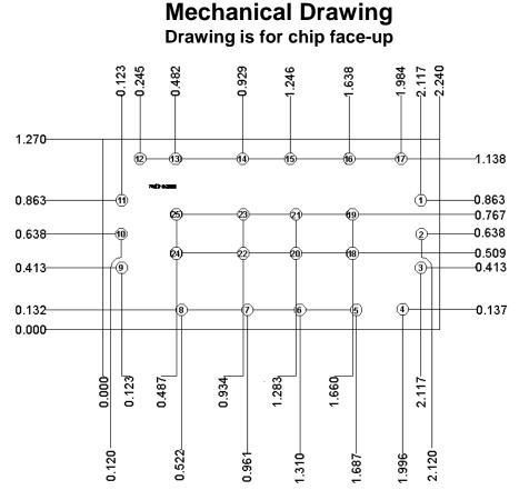
Units: millimeters Thickness: 0.380 Die x,y size tolerance: +/- 0.050 Chip edge to pillar dimensions are shown to center of pillar
