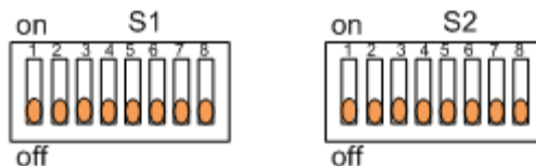
Figure 14: S1 and S2 configuration for external application control through USB
