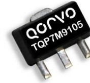
3-pin SOT-89 Package
