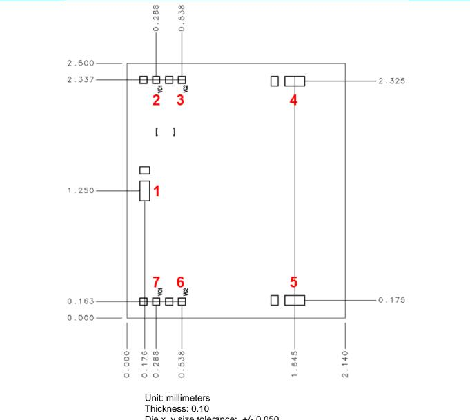
Die x, y size tolerance: +/- 0.050Chip edge to bond pad dimensions are shown to center of pad
