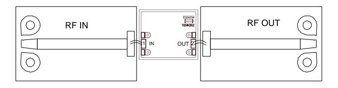
Note: RF Input and RF Output ports are not interchangeable.
