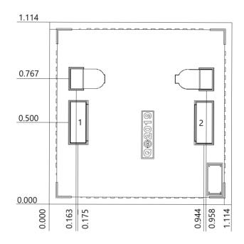
Unit: millimeters Thickness: 0.10
