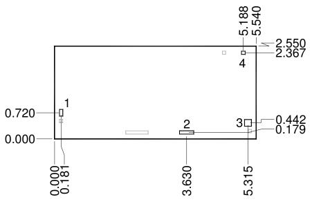
Unit: millimeters Thickness: 0.10 Die x, y size tolerance: ± 0.050 Chip edge to bond pad dimensions are shown to center of pad Ground is backside of die
