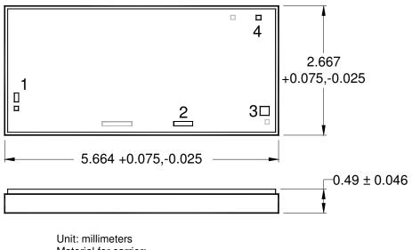
Material for carrier: Cu-Mo-Cu Thickness: 0.381 ± 0.025 Plating for carrier: Gold (Au) over Nickel (Ni) MMIC die is attached to carrier using solder MMIC die is nominally centered on carrier.
