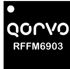
28 Pad 6x6 mm Laminate Package
