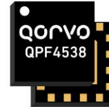
16-Pin, 2.5x2.5 mm Module Package
