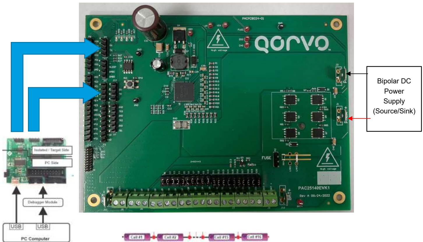
Figure 7: Evaluate PAC25140EVK with Cells Stack
