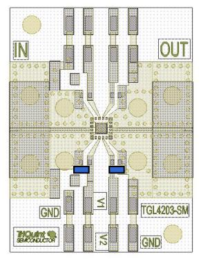
InF(size 0402) capacitors for DC decoupling Board material is 8 mil ROGERS RO4003
